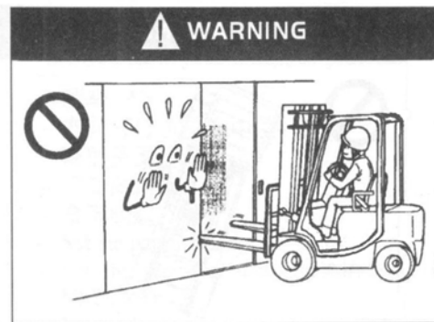
Do not abuse the forklift!
