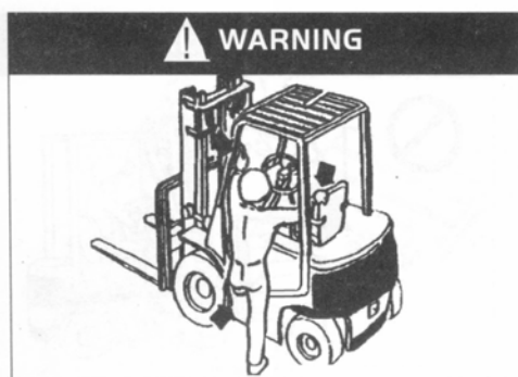
Hold the handrail during on-boarding
