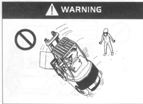
High speed during turning will cause workingoverturning due to unstable centre of gravity!
