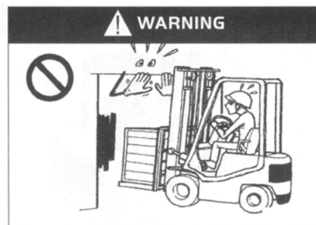
Always pay attention to the height of the working area of forklift!
