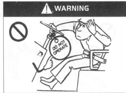
Do not drive an unsafe forklift!
