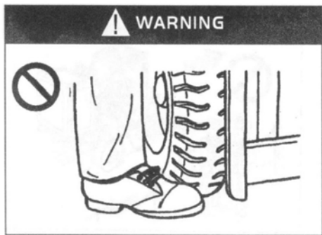
Please do not move the forklift when there are people standing in front of it!
