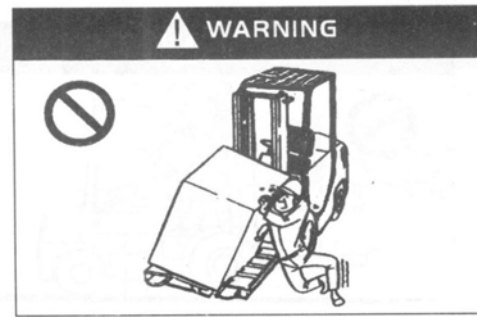
Do not carry damaged goods cases by your shoulders!
