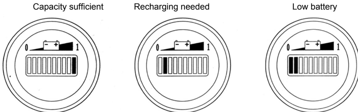
If the indicator shows low battery when lifting loads for a not very long period, lifting function can only be performed after recharging the accumulator to at least 70% of capacity.
