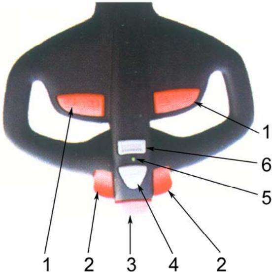
1. **Up/down switch:** Moving the fork upward or downward
